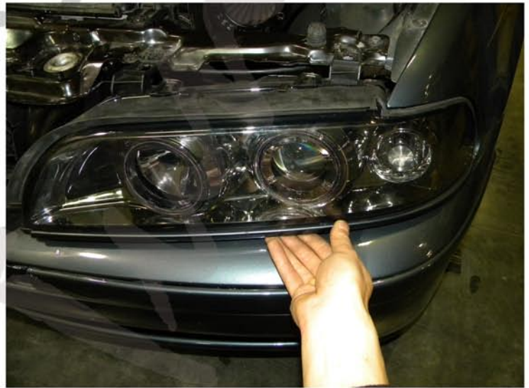
8. Remove the headlight
