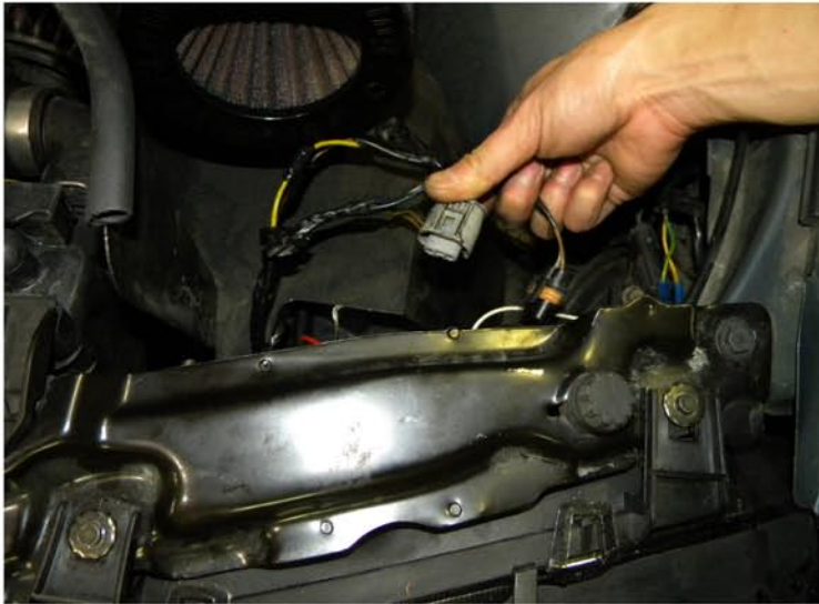
1. Disconnect the headlight harness
