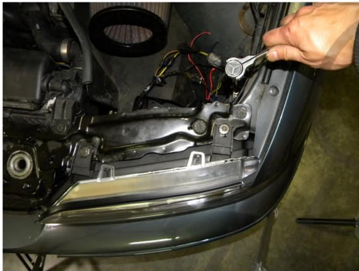
13. Tighten the (4) 8mm bolts
