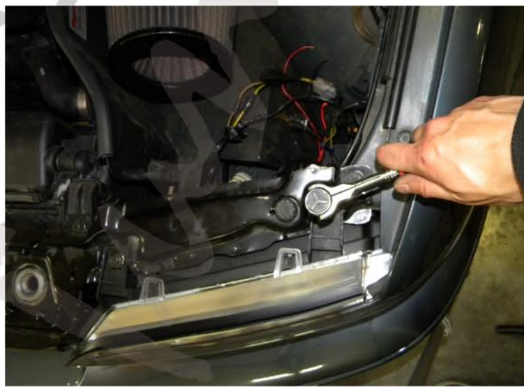
14. Tighten the (4) 8mm bolts
