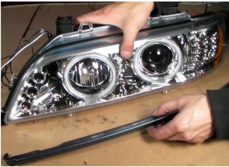
11. Place the painted trim on the new headlight
