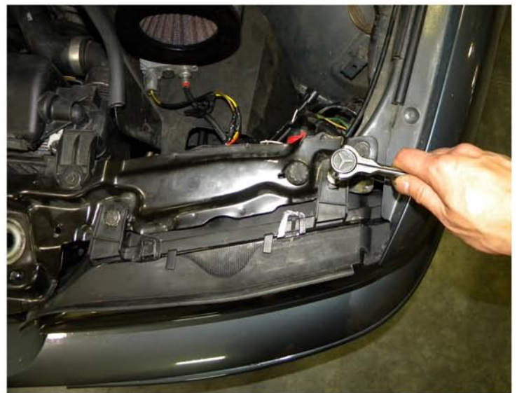
4. Remove the (4) 8mm bolts
