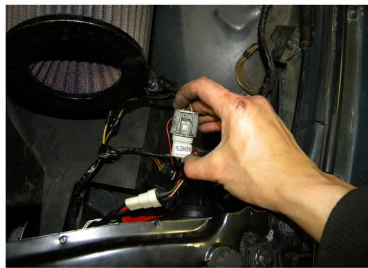
16. Connect the headlight harness to the new light
