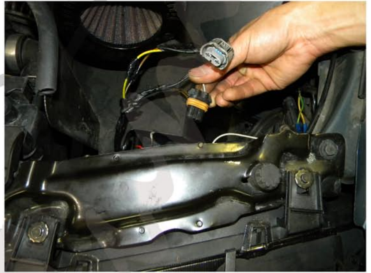
2. Disconnect the headlight harness
