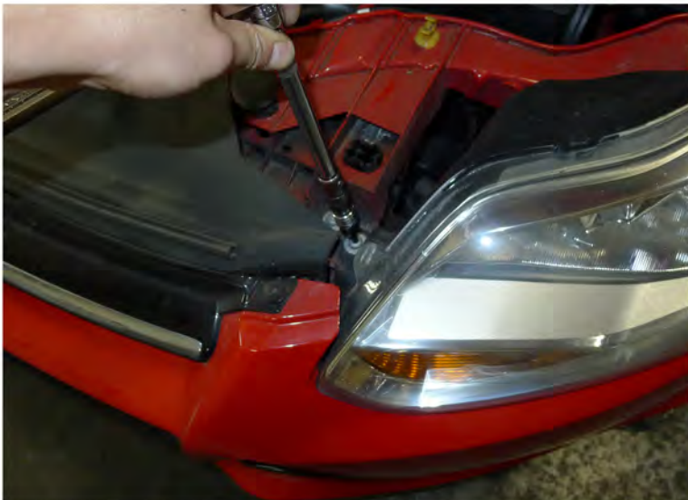
3. Remove the (2) T30 bolts
