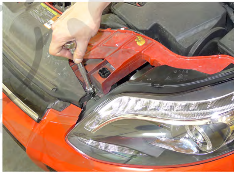
8. Tighten the (2) T30 bolts Please repeat the steps from 1 to 8 for the opposite side
