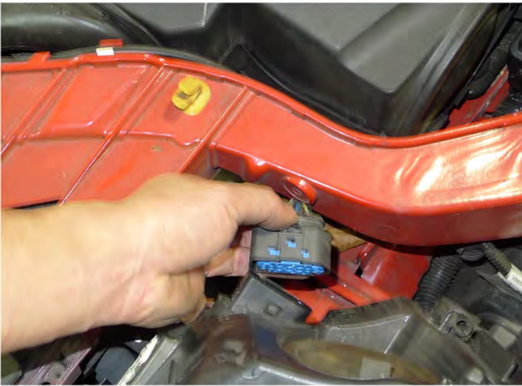
5. Disconnect the headlight harness and remove the headlight
