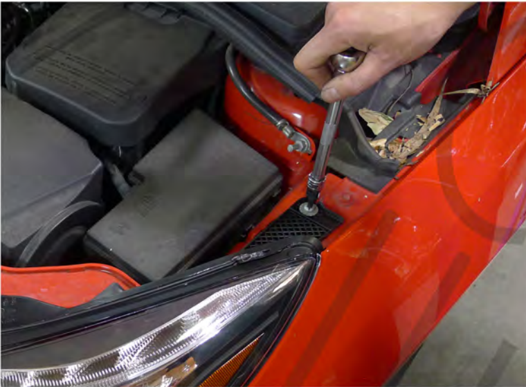
7. Tighten the (2) T30 bolts
