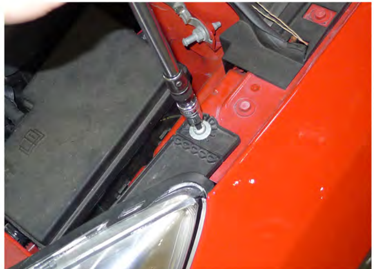
4. Remove the (2) T30 bolts
