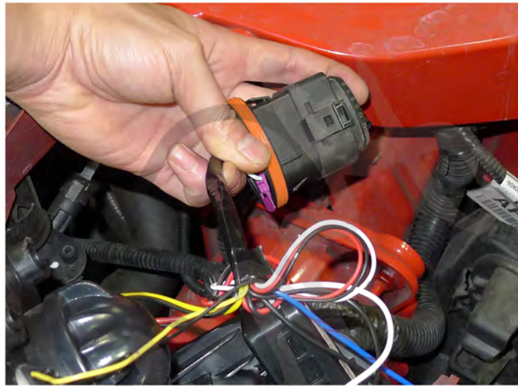
6. Connect the headlight harness to the projector headlight
