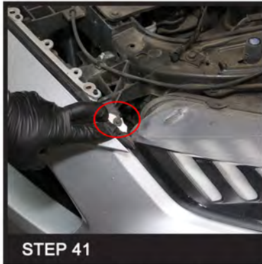
Reinstall the 7/32" bolt for both sides
