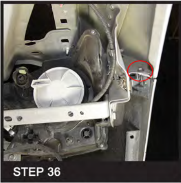
Reinstall the 7mm bumper mounting bolt for both sides
