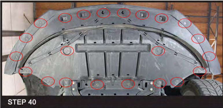
Reinstall the sixteen 7mm bolts and the six plastic clips
