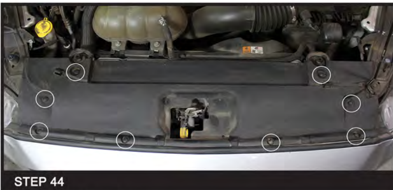
Reinstall the eight plastic clips
