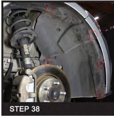
Reinstall the wheel inner liner and the five plastic clips for both sides
