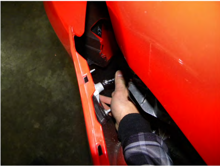
5. Unplug the bumper light bulb
