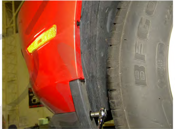
2. Remove the (2) 7mm screws
