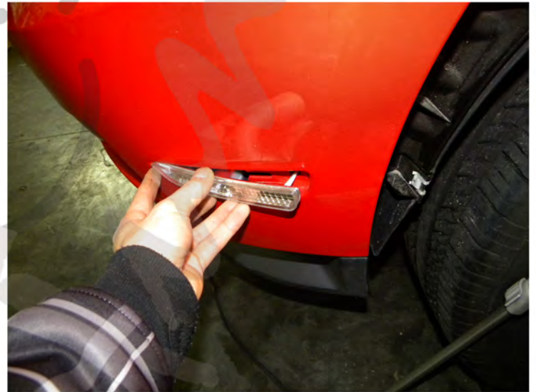
8. Place the new bumper light in the stock location
