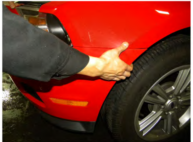
4. Pull on the side of the front bumper
