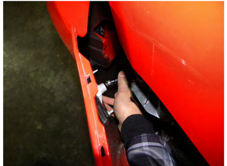
10. Plug in the bumper light bulb
