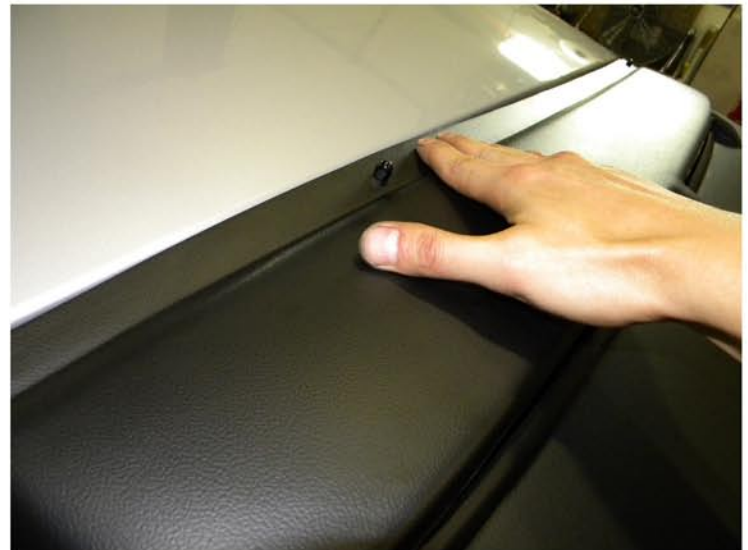
10. Press down on the mounting bracket to ensure the adhesion
