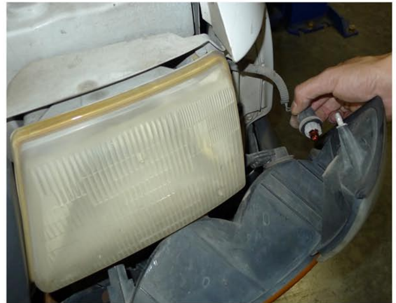
4. Disconnect the light sockets
