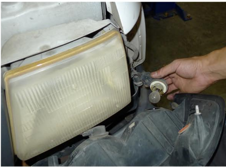
5. Disconnect the light sockets
