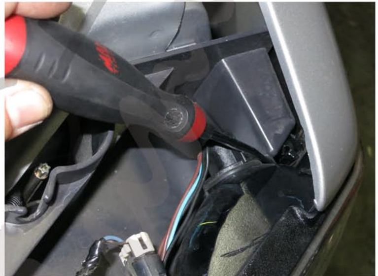
2. Release the retaining clip
