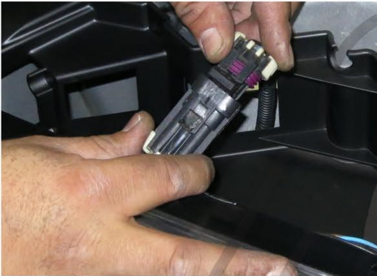
7. Connect the bumper light harness
