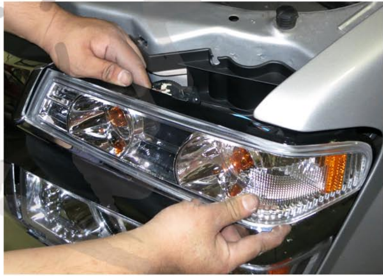
8. Place the new bumper light in the stock location
