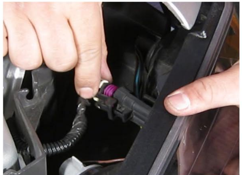
4. Disconnect the bumper light harness
