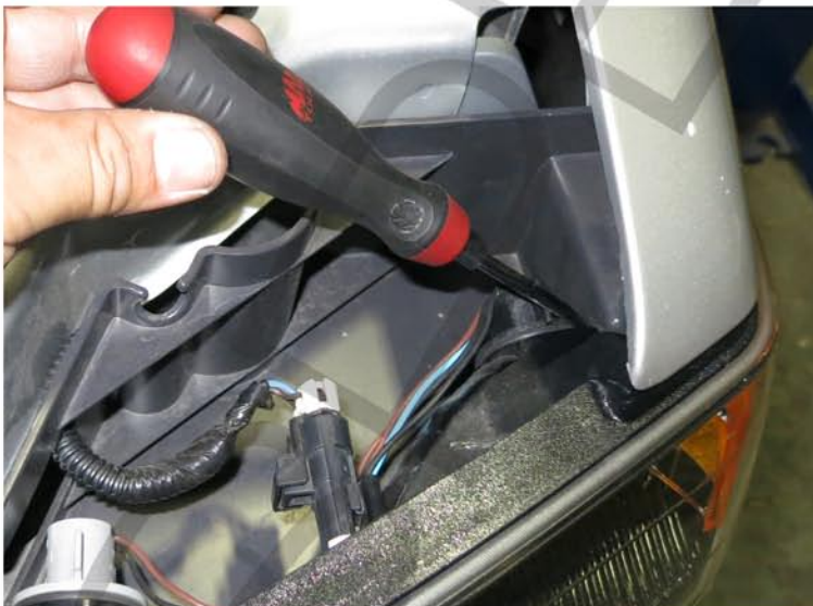
3. Release the bumper light retaining clip
