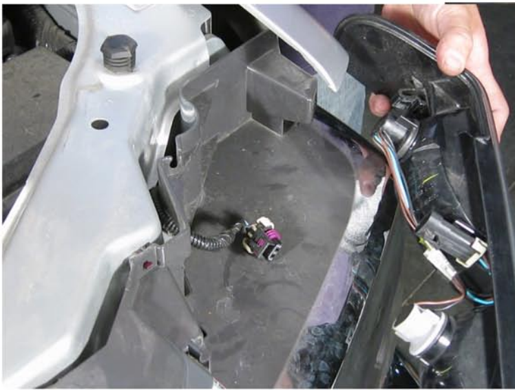
5. Remove the bumper light
