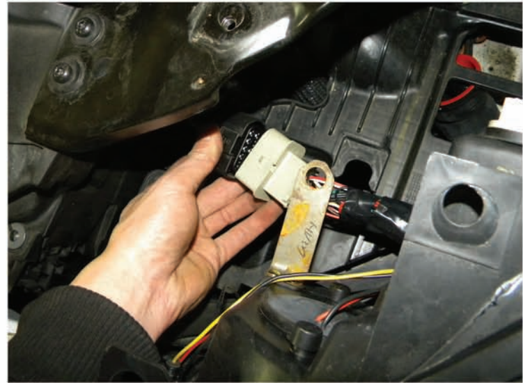
14. Connect the headlight harness onto the new headlight Please see the Halo and L.E.D installation instructions If your headlights don't have HALO or L.E.D. You can skip it
