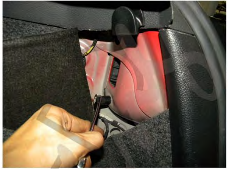
12. Install the new taillight and two 13mm taillight bolts
