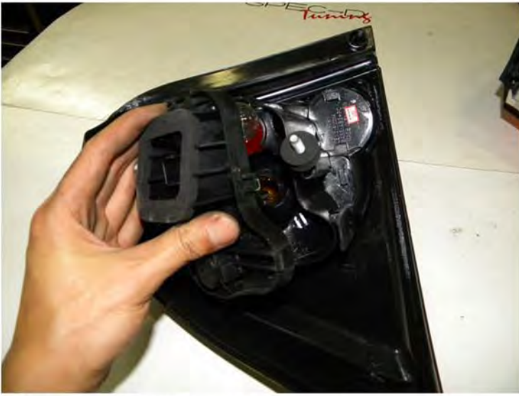
11. Install taillight socket to the new taillight
