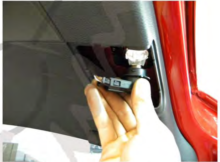
2. Remove back up light light bulb socket
