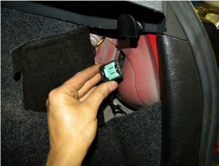
13. Connect the taillight harness please repeat the picture order from 1 to 13 for the opposite side
